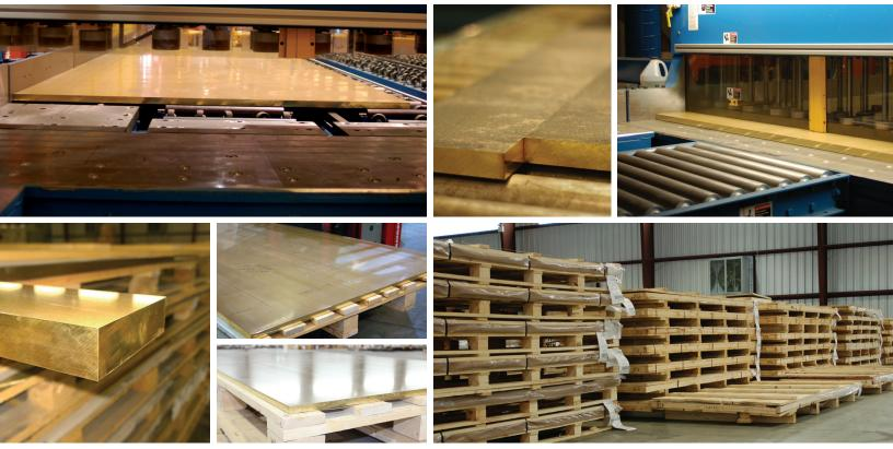
Aviva Metals maintains a large inventory of C26000 brass plate. C26000 70/30 plate is used more than any other brass product. It has excellent to good corrosion resistance in many applications, however it is not suitable for use with materials such as acetic acid, ammonia, hydrochloric acid and nitric acid.
